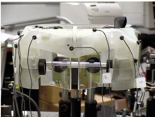
Figure 7. Realization of a Conformally Mapped Tracking Probe
