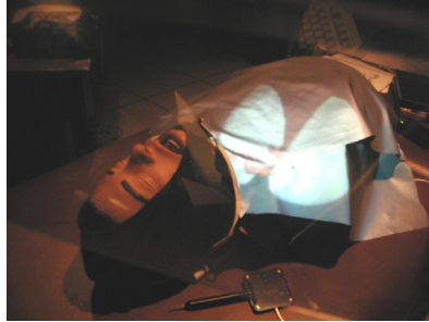
Figure 5. Trainee's view of the static lungs and trachea 3D models superimposed on the HPS
