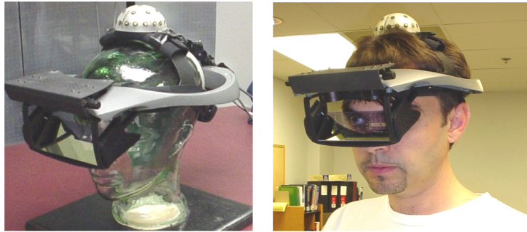
Figure 3. Optical see-through HMD and custom designed semispherical head tracking probe
