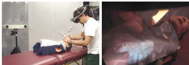
Figure 7. (a) Trainee and (b) trainee's augmented view filmed with a camera placed in place of one eye behind the HMD.
